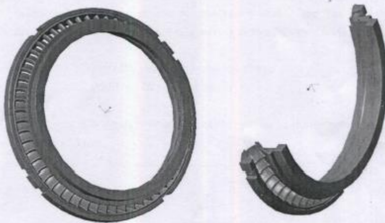
Figure: Stationary Blade Ring Complete and in Half part (Upper Part and Lower Part identical)
